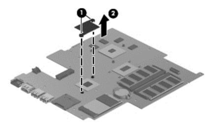
Reverse this procedure to install the PCH heat sink onto a replacement system board.
